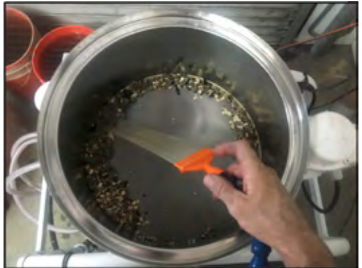
Figure 2. Sedimentary matrix washing using the electronic Sifter and attached water sprayer.
