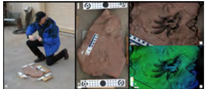
Figure 3. A. Hand-held, close-range photogrammetric documentation of selected specimens in the research collections at the New Mexico Museum of Natural History and Science (NMNHS) from PTNM was conducted in 2010 and 2018. B., Footprints of Dimetropus in the research collections at the NMNHS with coded targets for photogrammetry. C., Photogrammetrically processed image of Dimetropus track in Figure 3.B, showing orthophoto image with topographic contour lines (upper) and color depth map (lower). Contour interval 0.1 mm. Improvements in computer processing and photogrammetric software can be visualized when comparing the output products (Figure 2, C.D. and Figure 3C), as images taken in 2010 can be reprocessed with improved results over time.
