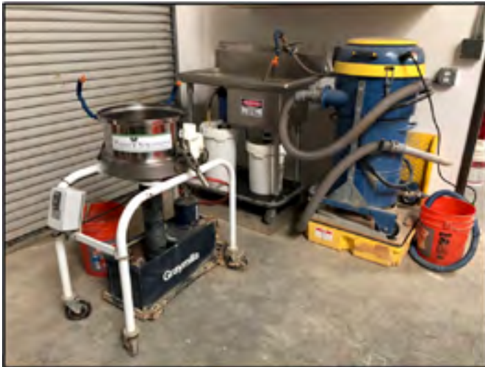
Figure 1. Complete sedimentary matrix washing set-up, including the electronic Sifter unit, water reservoir and water pump. Additional support equipment includes a self-contained and recirculating sink (the Qnk) and a shop vacuum.
