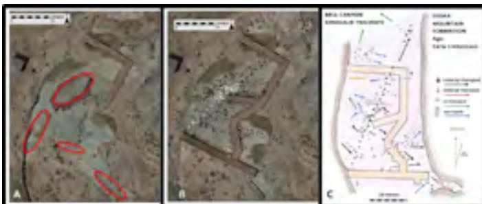
Figure 3. A., Composite stack of 2010, 2014, and 2017 orthophoto imagery. Of particular note is the expanded view of the track surface versus the small area initially available for study (circled in red), also of note is the virtual removal of a portion of the boardwalk. B., GIS track data is color-coded according to the area exposed in 2010 (depicted in light gray outlines) and overlain on 2014 orthophoto map. C., Ichnology map depicting selected trackways by MG Lockley. Note map is oriented to magnetic north.
